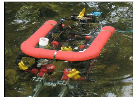
Figure 2. We placed a large ballast tank so that we could properly trim our ROV.
