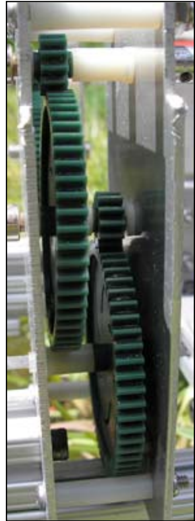
Figure 4. This is gear box we used on our claws.
