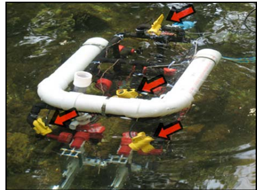
Figure 7. We strategically placed our black-and-white cameras so that we can have a good field of vision.
