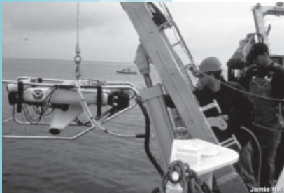
The crew of a NOAA oceanographic ship deploys a Phantom ROV during a research cruise in the Gulf of the Farallones National Marine Sanctuary. Photo credit: Jamie Hall
